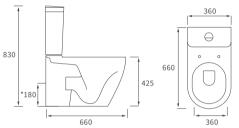
Coupling to soil stack: Straight out and straight down Distance from soil pipe spigot to wall: 250mm
