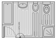
Undertile Wire System can be configured around any shape
