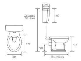
Coupling to soil stack: Straight out, straight down, Left or Right
