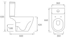
Coupling to soil stack: Straight out, straight down, Left or Right
