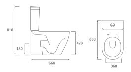
Coupling to soil stack: Straight out and straight down
